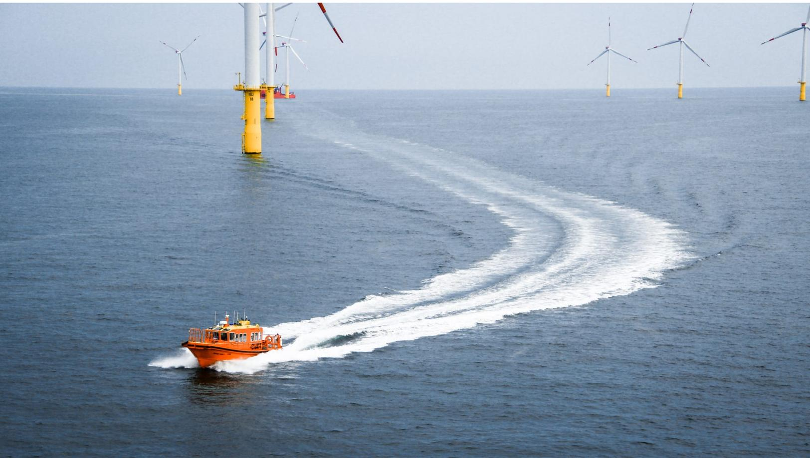
STB 12 is generally generously equipped. Everything on the vessel has full redundancy. As an example, there are two bow thrusters for full motor redundancy and for assistance with further manoeuvrability when mooring at the offshore wind turbine.
